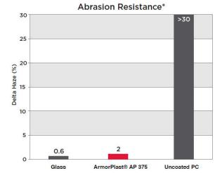
\*Taber Abrasion per ASTM D 1044, 100 cycles using CS-10F wheels at 500 g load
